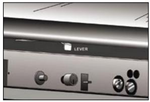
Figure 4. Venturi Adjustment Lever
